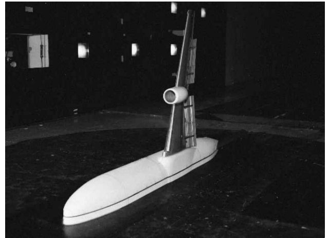
Fig. 2 Semispan EET model as tested with the 2-in., two-dimensional standoff in the 14 by 22 ft Subsonic Tunnel.
